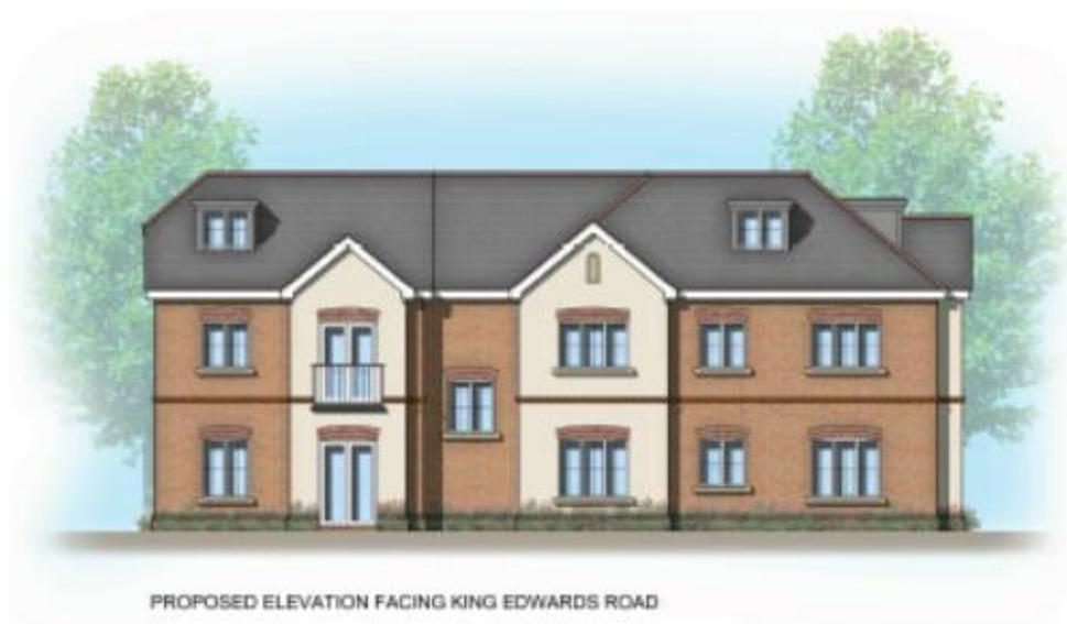
9.42 The design of the building would replicate that of the flatted development to the north-west of the site at Drummond Court in relation to a similar roof design comprising hips, gables and dormer windows and materials comprising a mix of render and brick. Architectural detailing would include soldier courses above windows and doors and brick stringcourse to add design interest to the building.
